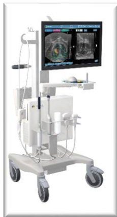
Fusion platform Navigation + Software to fuse MRI+US
